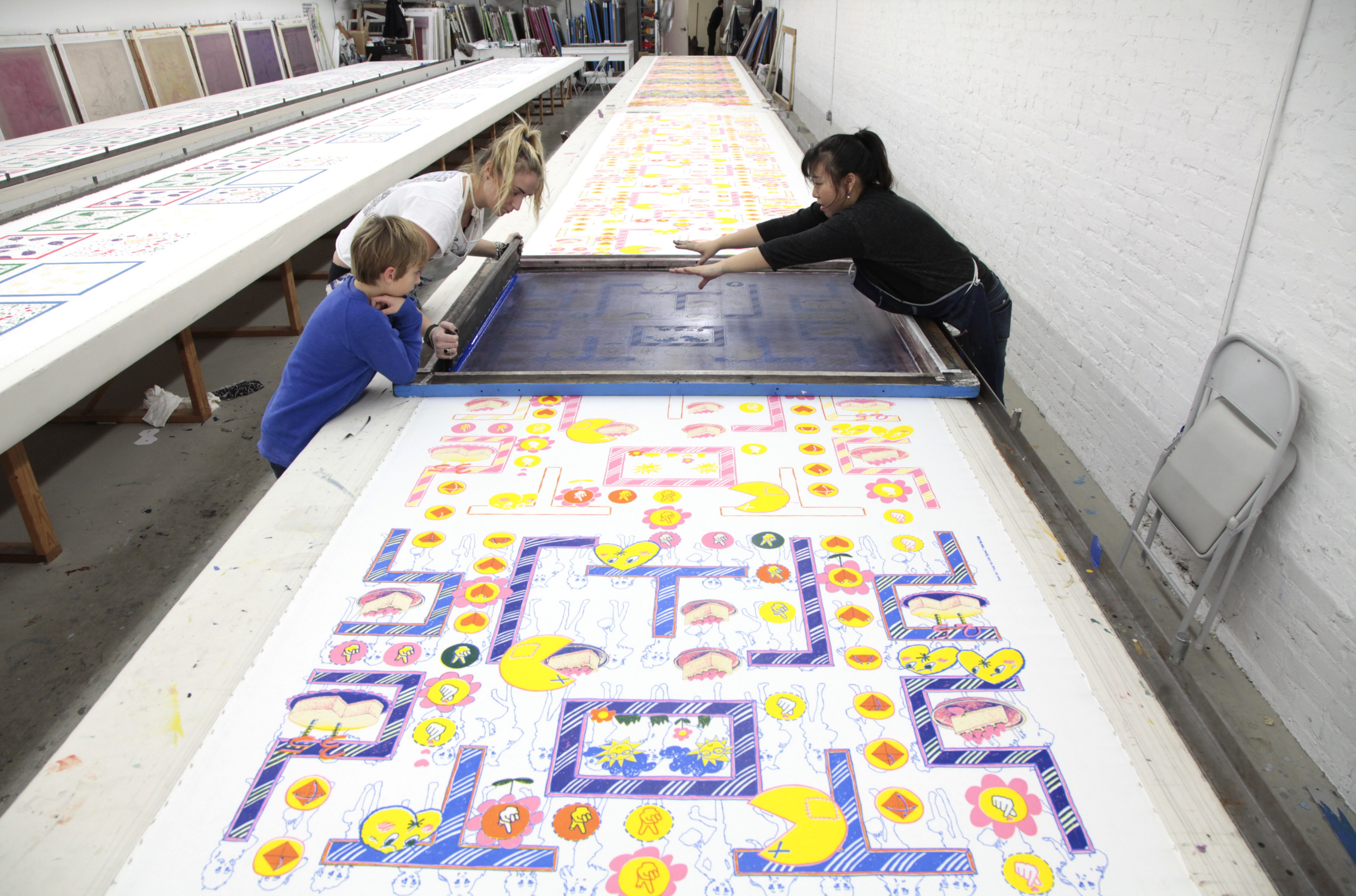
Screenprinting a repeat pattern on fabric
