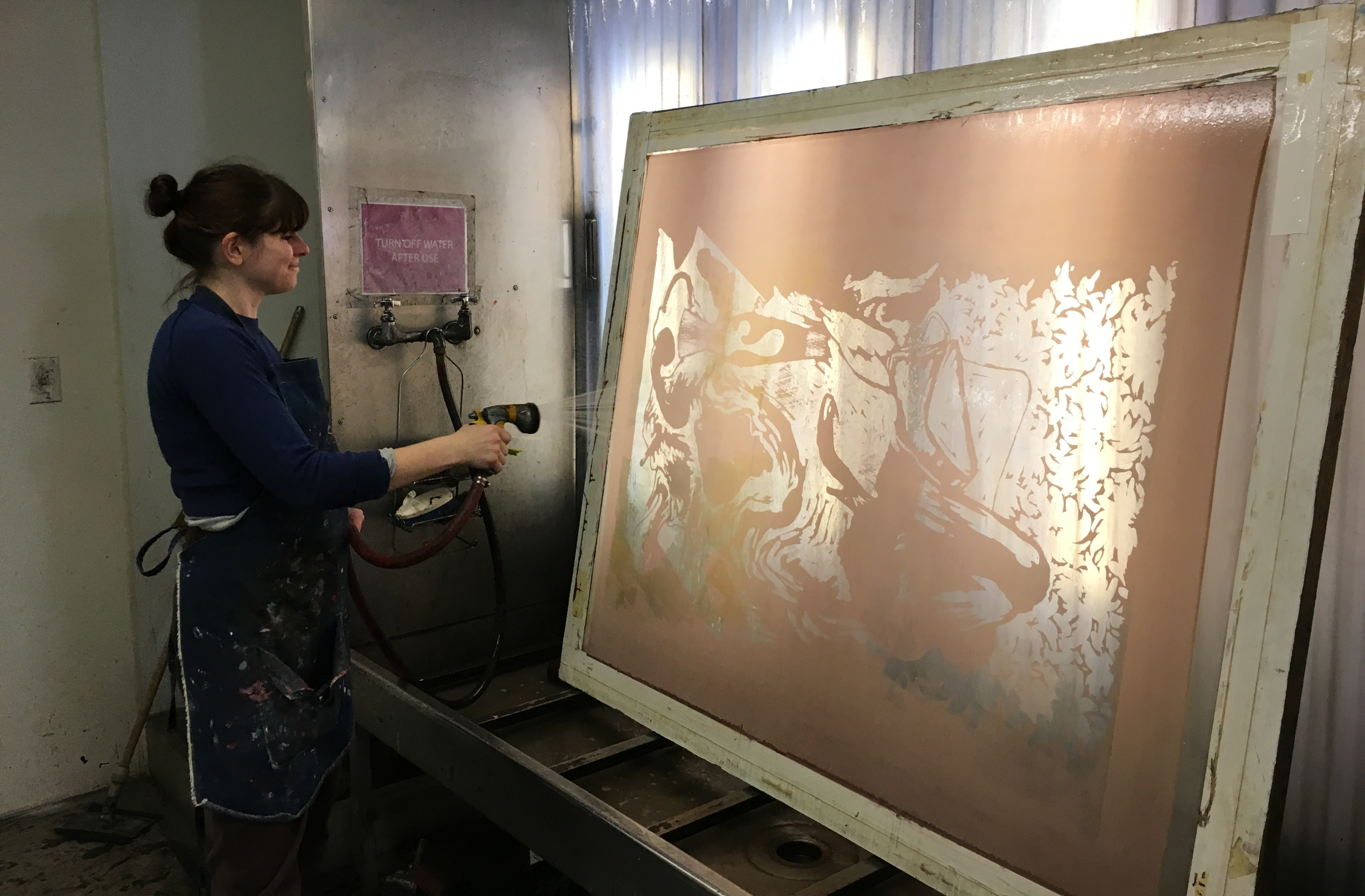
Washing out an exposed screen
